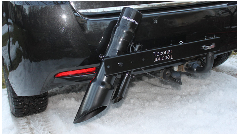
Figure 4.1: A Teconer RCM411 sensor system [26] attached to a car (image source https://www.teconer.fi/en/surface-condition-friction-measurements/#RCM411 ).
