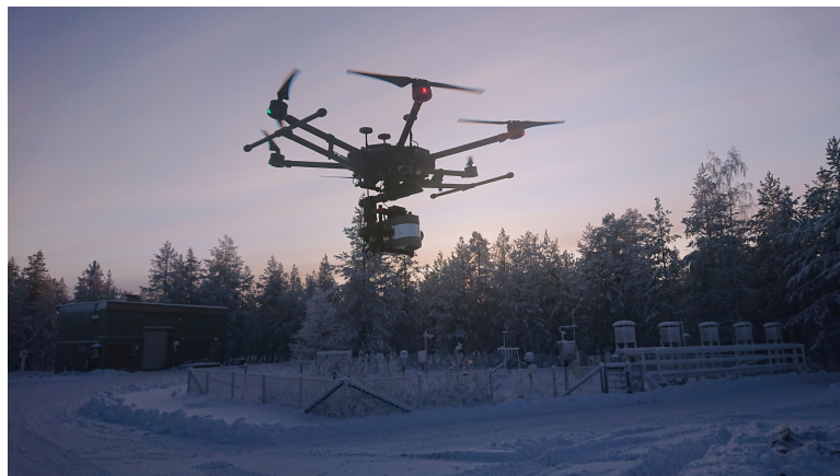
Figure 4.2: An FMI DJI Matrice 600 Pro UAV [1] in flight on 30 Oct 2019 in Sodankylä. The payload is a Rikola hyperspectral camera. Photo: A. Rimali/FMI.
